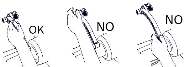
Fig. 100: Correct handling of the electronic rim-distance gauge
