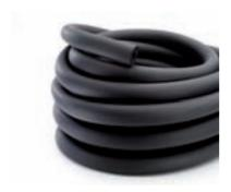
Flexible rubber pipe insulation with the same insulation properties as INSUL-TUBE® K. The product is rolled up in a practical dispenser. This enables insulation of continuous long pipes with minimum time spent cutting and gluing.
