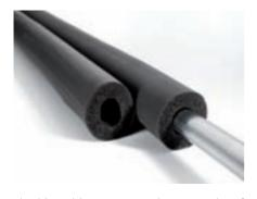
Flexible rubber pipe insulation made of closed-cell foam for refrigeration and air conditioning systems. The closed-cell structure and good water vapour diffusion resistance of the material prevent condensation from forming on cold pipes and guarantee durable energy savings.
