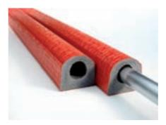
$\mathsf{EXZENTROFLEX}^{\mathsf{@}},$  the solution for small floor panel thicknesses. The excentric, extruded polyethylene pipe insulation with robust PE-shell for insulating floor pipes, in accordance with the German Energy Saving Act (EnEV), offers high tilt stability due to its design.
