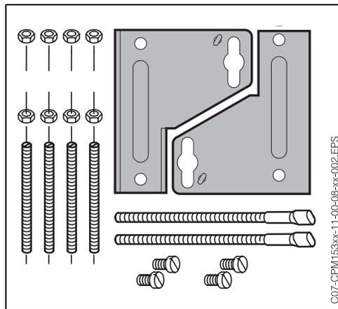
Mounting the transmitter in panels or on posts CPM 153 using supplied mounting kit (see left).
