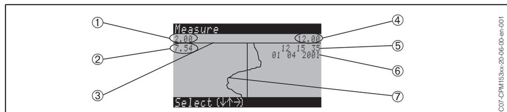
Example for data logger (for Parameter 1, pH is selected here)
