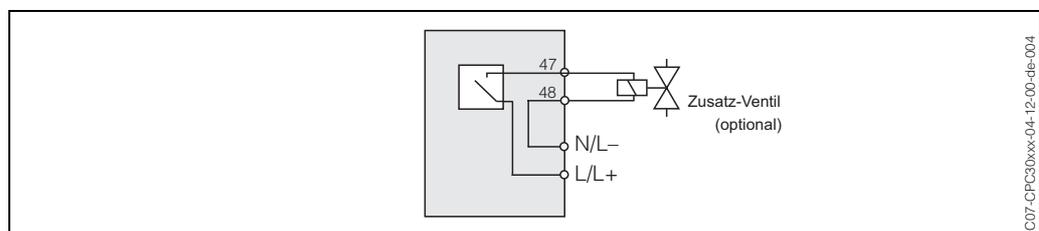
Switched mains voltage to control the additional external valve
