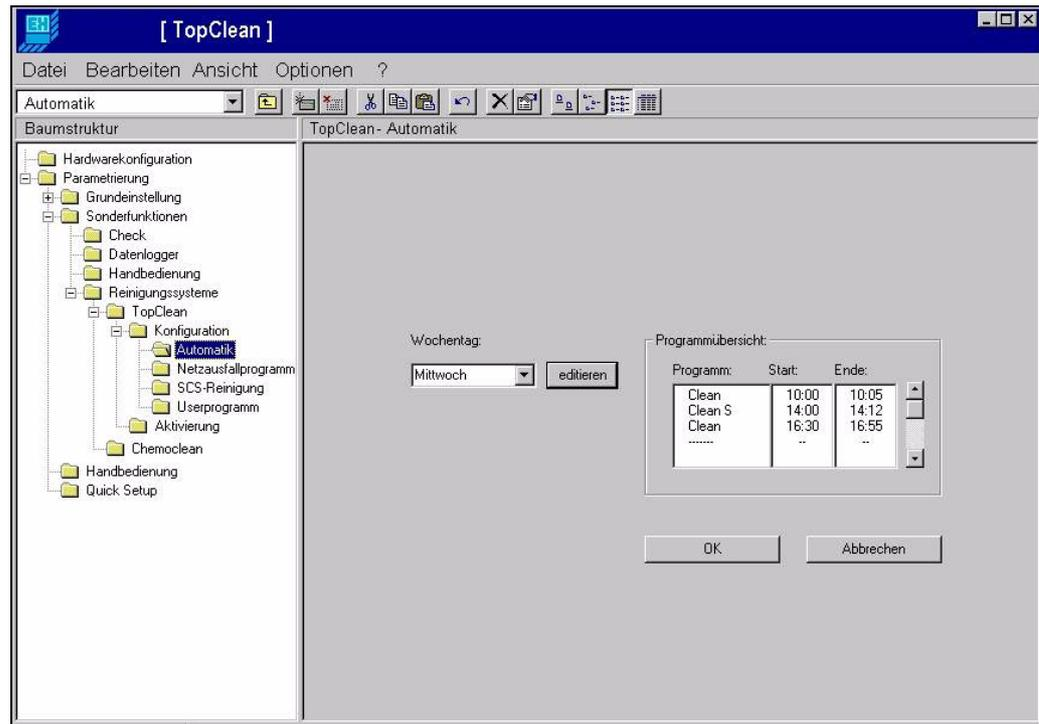
The PC tool Parawin provides you with a tool for configuring your measuring point on a PC using a simple and self-explanatory menu structure (an example window can be seen above). Write the configuration to the DAT module using the RS232 interface on the PC. The data can then be transferred to the transmitter.
