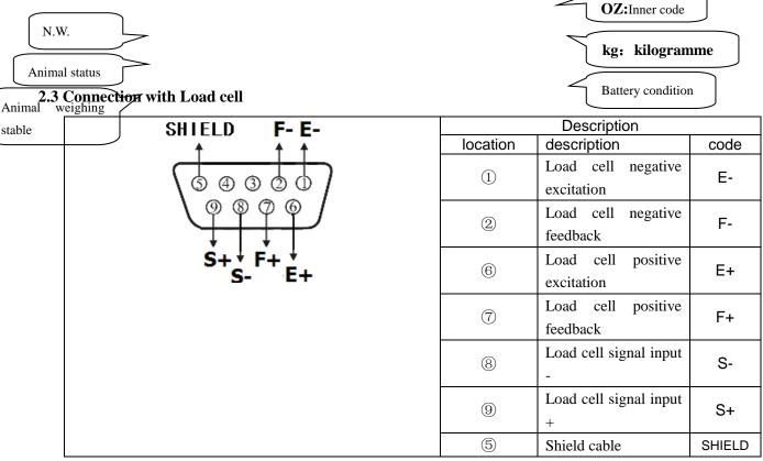
This indicator is connecting with 4 wires cable, user must make the short circuit for positive excitation and positive feedback negative excitation and negative feedback
