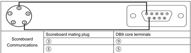
▲! The connection between scoreboard and indicator scoreboard output must be correct, if with wrong connection, it will cause damage to output interface of indicator or input interface of scoreboard .Even it will damage seriously indicator and scoreboard . Special connection cable shall be used. The scoreboard will display nothing when the indicator is under calibration status.
