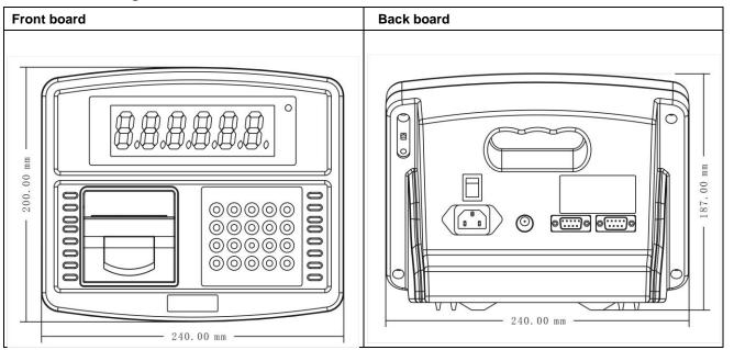
Remark: The 9 hole interface at back is for connection with load cell,9 pin interface is for scoreboard connection.
