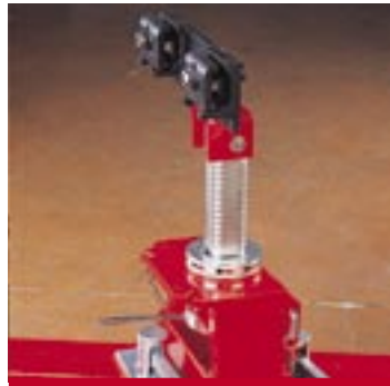
Column with anchoring clamp.
