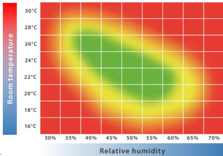
This „feel comfortable“ chart for indoor room climate demonstrates the combination of relative humidity and room temperature where the overwhelming majority feels comfortable in indoor rooms.
