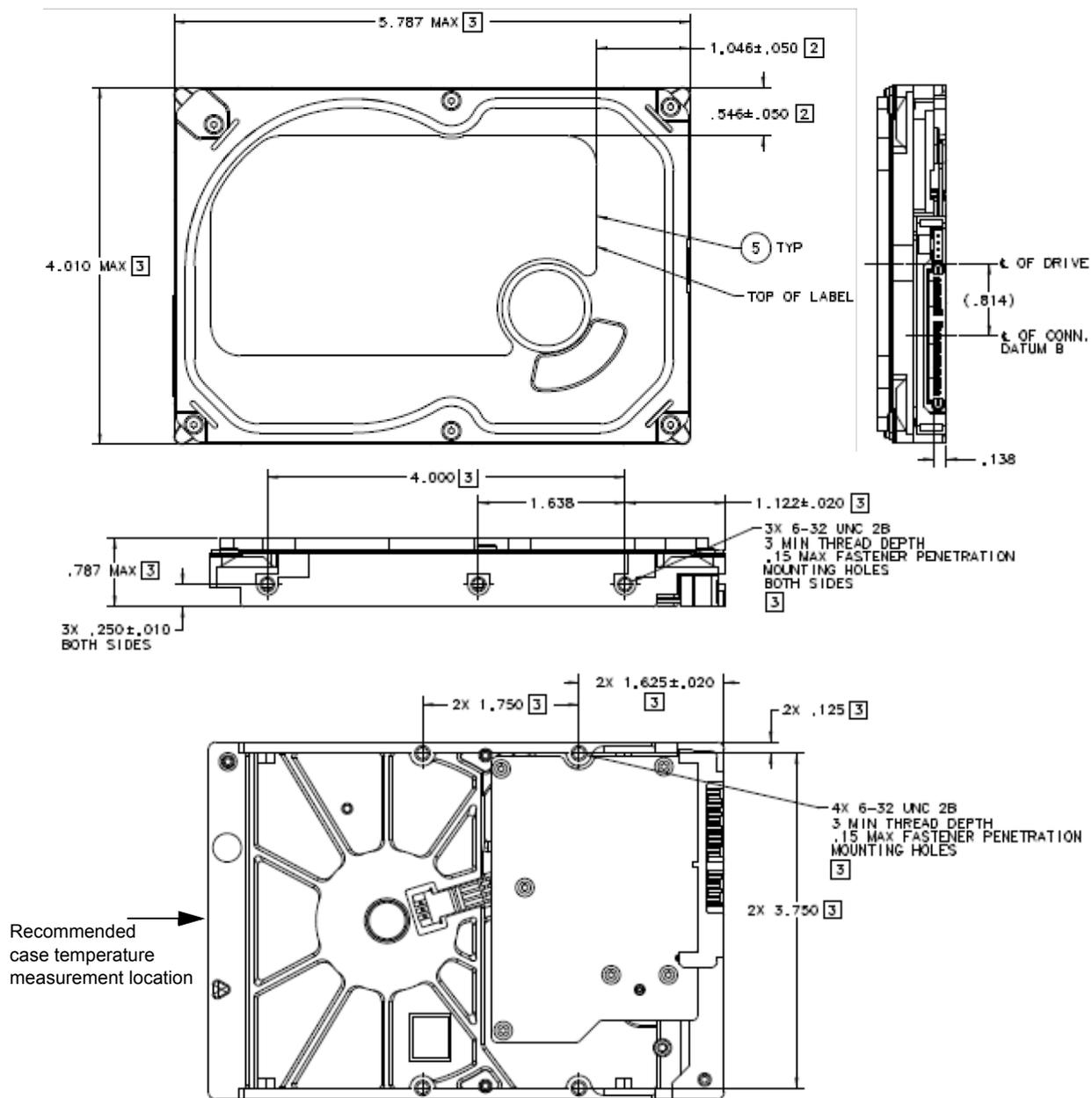
Figure 4. Mounting dimensions (for 500, 320, 250 and 160GB models)
