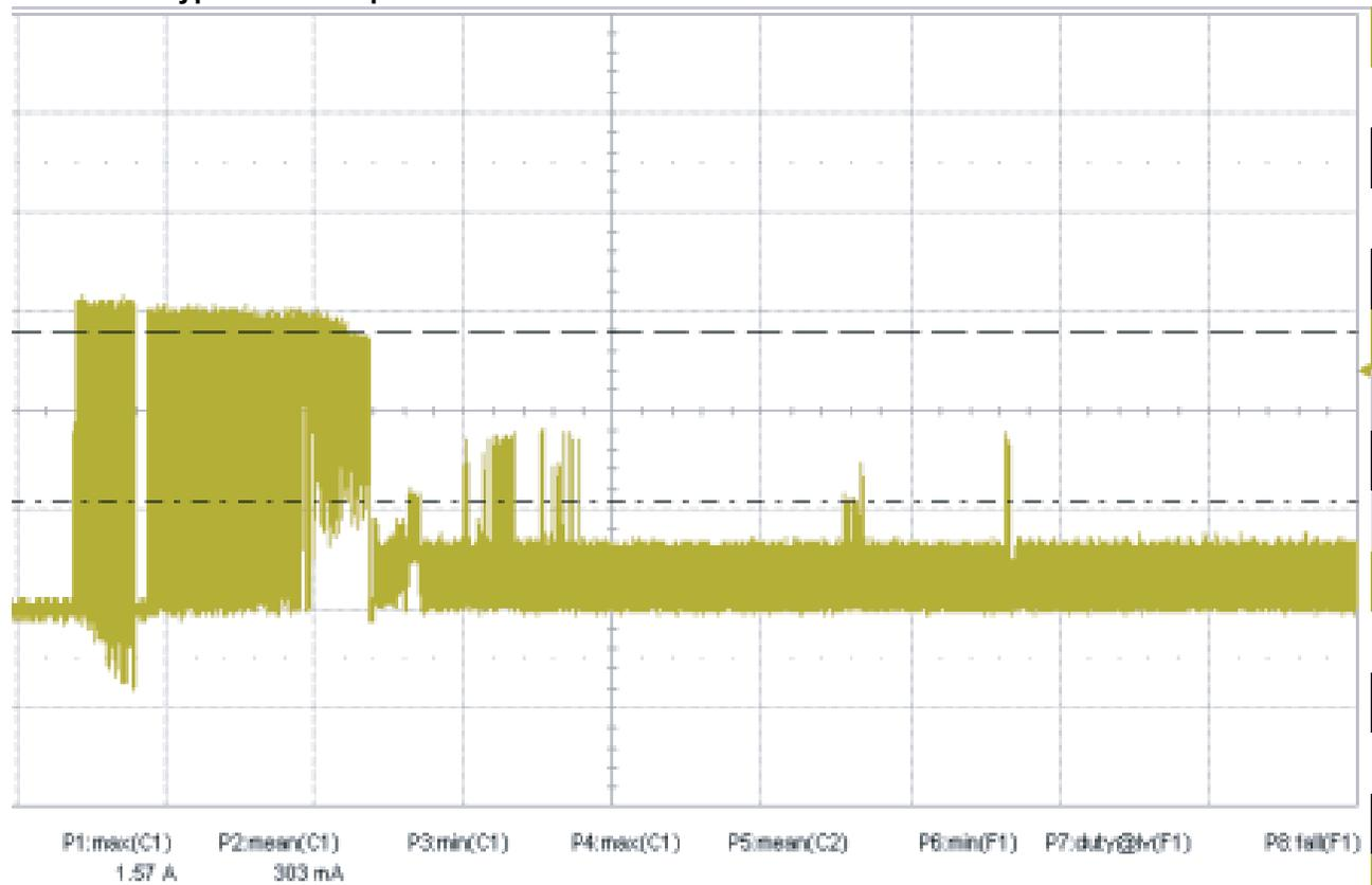
Figure 1. Typical 12V startup and operation current profile
