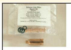
**LINE FILTER** Use Delavan's line filter for extra filtration in burner applications of 2.00 GPH or less. These offer four times the filtering area of a standard nozzle stainer and twice the protection. A plugged line filter can cause a pressure drop. Check the pressure on the outlet side of the filter while the unit is flowing to see that it is the same as the pump pressure. If less, replace filter.
