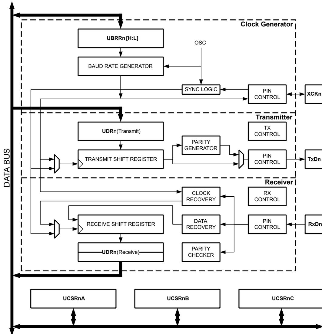
**Note:** Refer to the *Pin Configurations* and the *I/O-Ports* description for USART pin placement.
