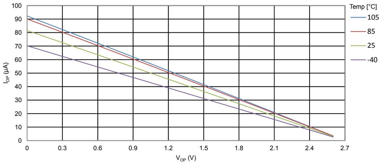
**Figure 34-18. ATmega328PB: I/O Pin Pull-up Resistor Current vs. Input Voltage ( $V_{CC} = 5V$ )**
