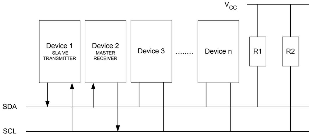
To initiate the SR mode, the TWI (Slave) Address Register (TWARn) and the TWI Control Register (TWCRn) must be initialized as follows:
