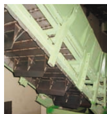
■ Special model at a trimming shear with a belt width of 900 mm
