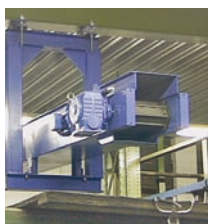
■ Hinged belt conveyor for loading of a hopper system
