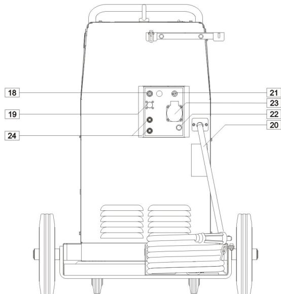
18. **Socket:** For connecting gas supplying hose.
