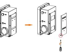
STEP 2: Fix the back bracket and the cable hook (only for type P) to the wall.
