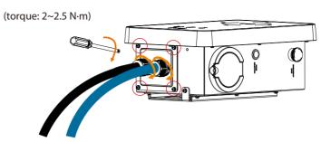
STEP 12: Hang the EV-Charger up carefully and steady the EV-Charger with the self tapping screw and the cross screwdriver.
