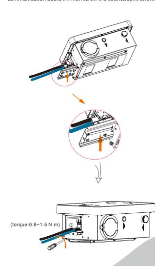
STEP 11: Push the rear cover to appropriate position of the cables and screw the self tapping screws with the cross screwdriver. Then tighten the waterproof fastening head.
