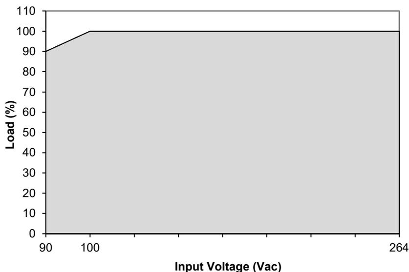
**Fig. 2 De-rating for AC Input Voltage**
