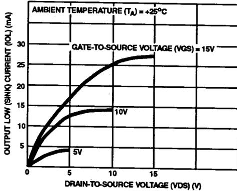
FIGURE 3. TYPICAL OUTPUT LOW (SINK) CURRENT CHARACTERISTICS
