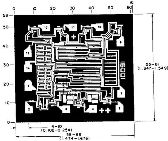
Dimensions in parenthesis are in millimeters and are derived from the basic inch dimensions as indicated. Grid graduations are in mils ( $10^{-3}$  inch).
