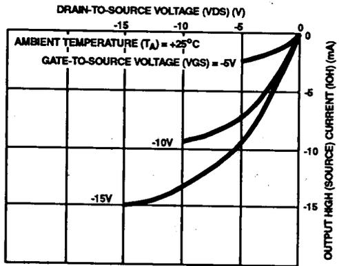
FIGURE 6. MINIMUM OUTPUT HIGH (SOURCE) CURRENT CHARACTERISTICS
