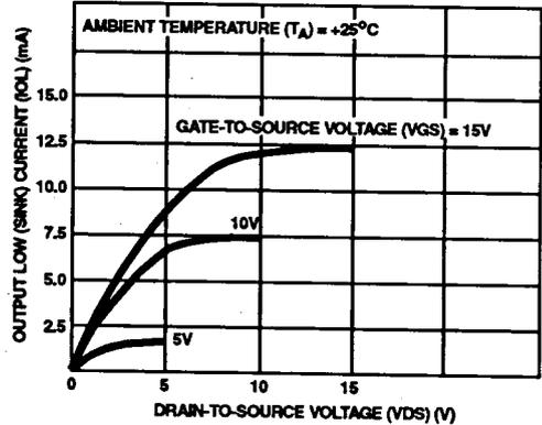
FIGURE 4. MINIMUM OUTPUT LOW (SINK) CURRENT CHARACTERISTICS
