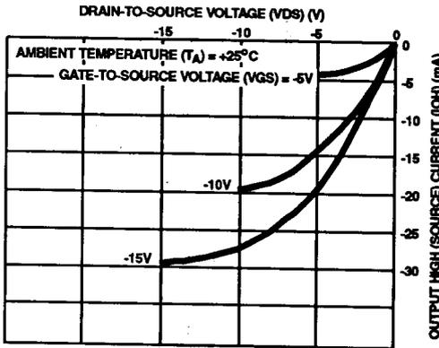
FIGURE 5. TYPICAL OUTPUT HIGH (SOURCE) CURRENT CHARACTERISTICS
