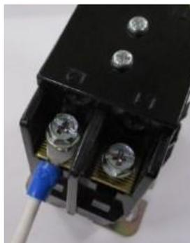
Figure 24: Wiring 220V Contactor
