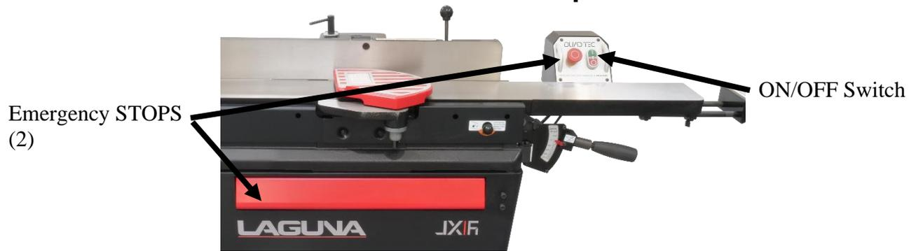
Figure 7: Control Panel & E-STOPS
