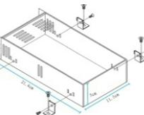
Notes: Please use our screws only since it may damage the internal PCB if using other screws. Please use proper torque to push the screws into casing since it may damage the internal PCB by strong torque.
