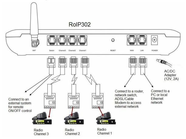
a. Connect the Switch Port to an external system for remote control. It can be used to switch onand off a Public Announce (PA) system to instant broadcast. If the relay switch is connected to high voltage load. The maximum rating for the internal relay is 240VAC and 500 mA load current.
