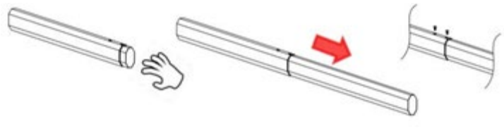
Figure 1 Connect the main boom with the Secondary arm together by 2 screws
