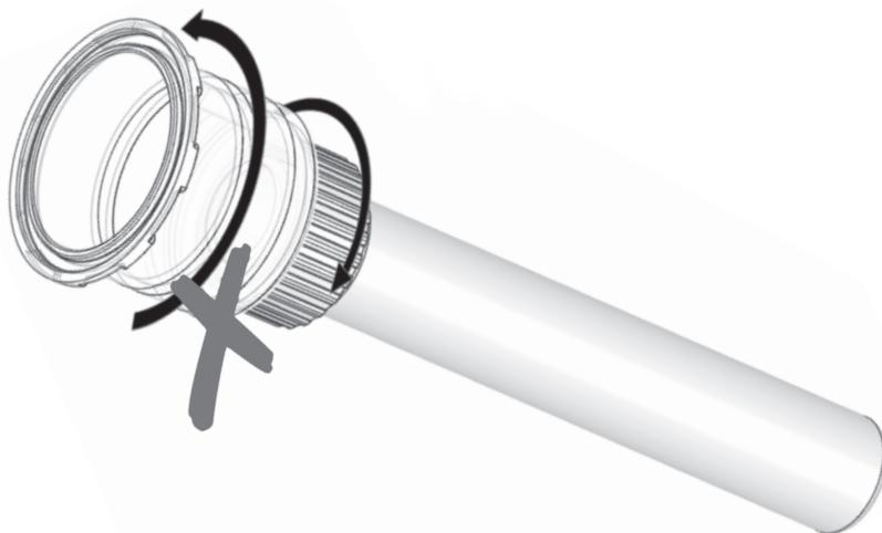
**EN: Do not disassemble!** The quartz glass connection cannot and may not be dismantled.
