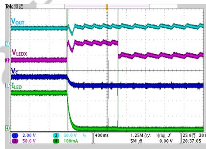
**Electrolytic capacitor short test**
