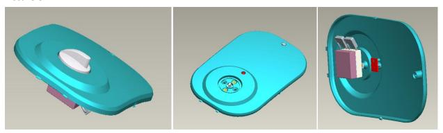
2. **Disassembly of thermostat (picture 3)----** After removing the maintenance cover, detach the knob with pliers; using air screw or screwdriver to remove screw (M4X10) and pulling out the inner wire assembly terminal, then pull out the sensing temperature probe from the heating pipe of heating element.
