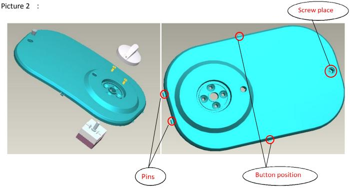
1. **Disassembly of maintenance cover (picture 2)----** Maintenance cover is assembled through 2 pins, 2 buttons and 1 tapping screw with top cover. When disassemble it, firstly to use an awl to open the screw cap. Then using the air screw or screwdriver to unscrew the cross round head tapping screw. After that, the maintenance cover can be detached.
