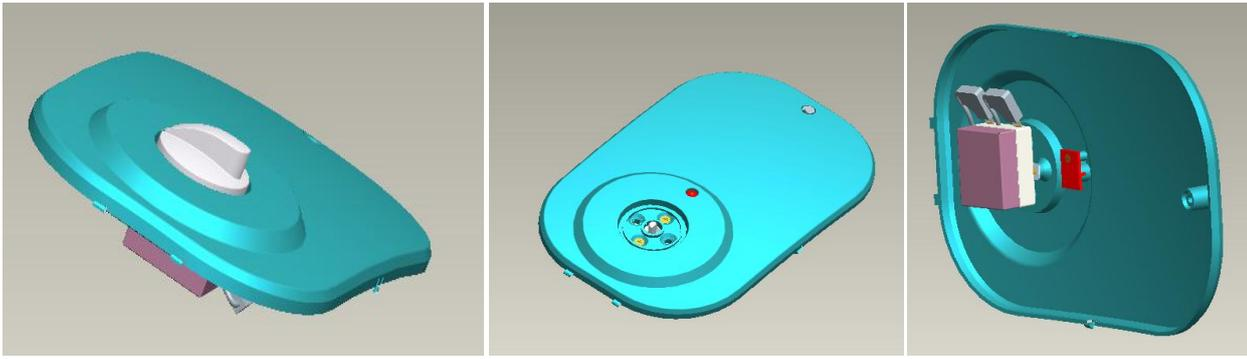
2. **Disassembly of thermostat (picture 3)**----- After removing the maintenance cover, detach the knob with pliers; using air screw or screwdriver to remove screw (M4X10) and pulling out the inner wire assembly terminal, then pull out the sensing temperature probe from the heating pipe of heating element.
