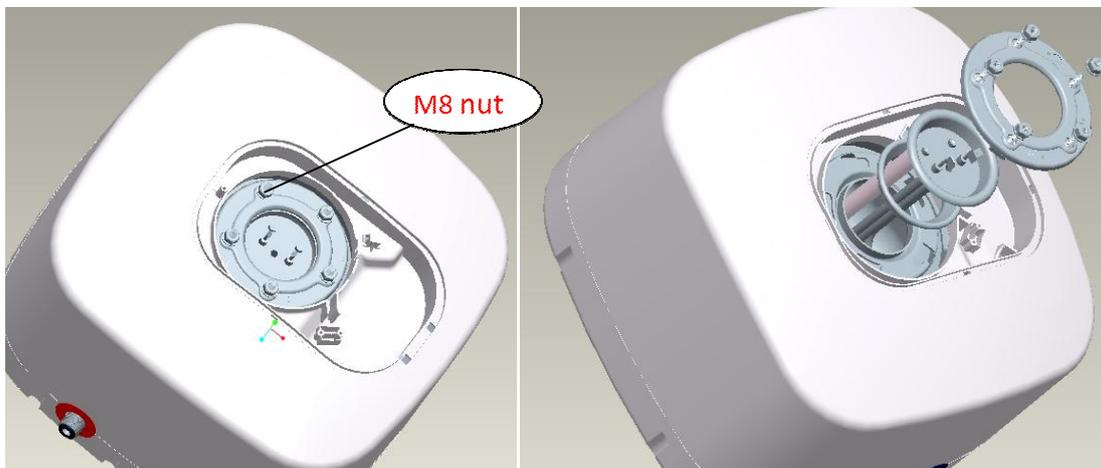
3. **Disassembly of heating element (picture 4)**----using air screw or screwdriver to remove 2 screws which lock the temperature limiter and remove it; then remove the nut that lock heating element, pulling out the inner wire assembly terminal from heating element , then heating element can be taken out directly.
