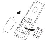
Each time when insert the batteries in the remote controller for the first time, you can set the Cooling only or Heating pump control type. As soon as you insert the batteries, turn off the remote controller, and operate as below.
