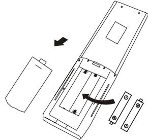
⚠ Each time when insert the batteries in the remote controller for the first time, you can set the Cooling only or Heating pump control type. As soon as you insert the batteries, turn off the remote controller, and operate as below.
