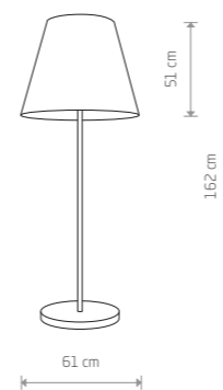
MOSS fabric, plywood, painted steel
