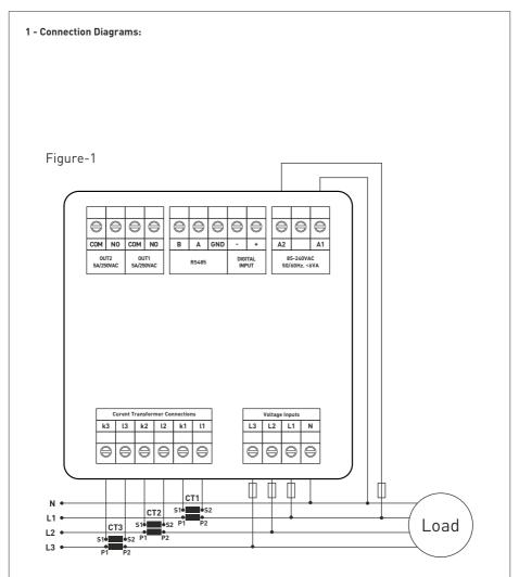
Figure-1: 3P4W connection type: 3 phase current and 3 phase voltage and neutral.
