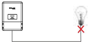
Incorrect Connection between Load and Inverter
