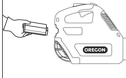
To remove the battery pack, lift up on the battery release, grasp the sides of the battery pack and remove it (Fig. 10).
