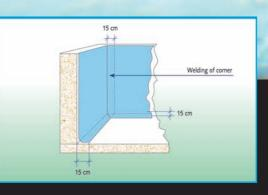
If the fitter so chooses, angular 90° corners or rounded forms with a radius of around 15 cm can easily be made. These extra lengths are generally allowed on the breadthwise panels. The corner should therefore be made on that extra length.
