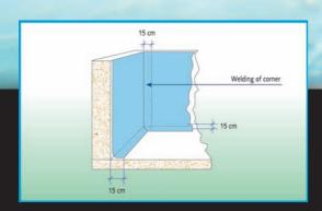
If the fitter so chooses, angular 90° corners or rounded forms with a radius of around 15 cm can easily be made. These extra lengths are generally allowed on the breadthwise panels. The corner should therefore be made on that extra length.
