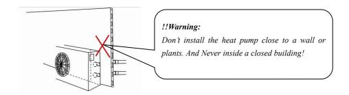
2. The heater should be located in a solid, level and non-corrodible structure that is capable of supporting the weight of the heat pump. It must be fixed by bolts (M10) to concrete foundation.
