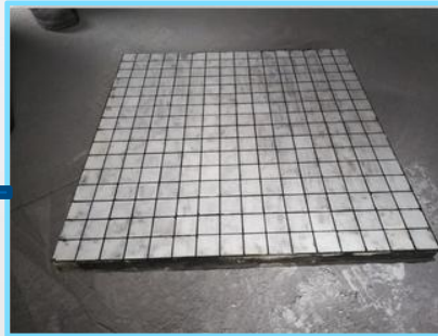
4. Put it into the vulcanization machine to vulcanize
