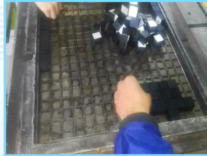
2. Put the ceramics into the steel frame
