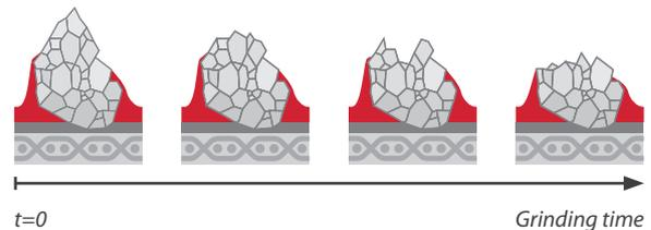
The microcrystalline structure of the **VSM CERAMICS** series enables a much more subtle breaking down of the grain and constantly produces new sharp edges.
