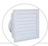
White PVC shutters feature full-length spring steel rods instead of plastic pins in the ends which lock into a heavy PVC frame with reinforced corners. True airfoil shutter vanes reduce air drag. \*This shutter is included with the fan
