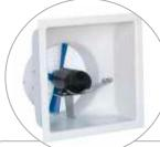
A high service factor 1/2 HP motor powers the AirStorm 36" fan. The high S.F. rating provides protection from motor failures caused by varying rural electrical voltage. Stainless steel motor mounts and hardware provide superior corrosion resistance.
