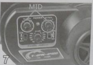
Adjust the throttle, steering vernier adjustment knob button to median (MID) direction .big/small rudder Angle knob button to 120%
