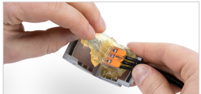
Simply extend circuits: Open the Gelbox, remove gel from the connector, open the connector and connect new components to the cable.
