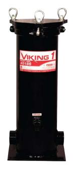
VIKING 1 PART # 40186 UP TO 120 GPM 2" NPT IN/OUT 12" DIAMETER 32.5" LENGTH 1 ELEMENT
