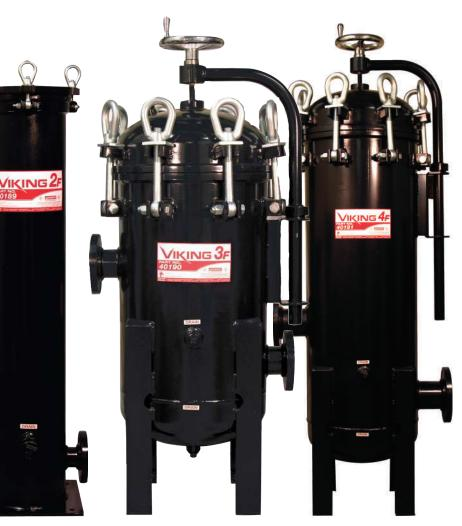
VIKING 3F PART # 40190 UP TO **300 GPM** FLANGED IN/OUT 3" RFSO FLANGE 24" DIAMETER 59.25" LENGTH **4 ELEMENTS**
