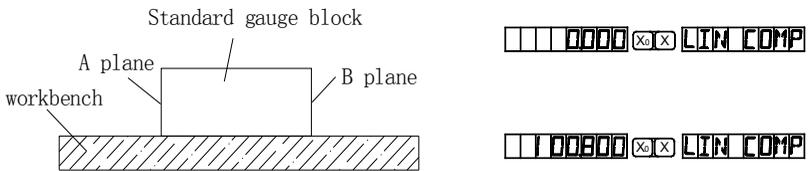
3. Move X axis to align with the B plane, press the " $\boxed{ENT}$ " key, deputy window will show "SET OK", then the linear compensation of X axis finished
