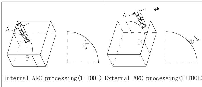
Milling cutter may be flat-bottomed or arc-bottomed. If flat-bottomed, set the tool diameter as 0;
