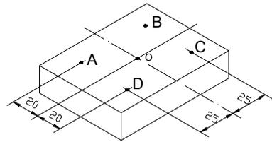
As the figure showed right, center point is the datum of ABS, the position of point A, B,C, D is (-25, 20), (25, 20), (25, -20), (-25, -20) in ABS coordinate.
