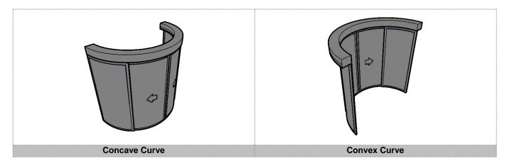
These type of doors enable wind-breaking and/or airlock installations (2 semicircular doors making up the entire diameter). Even though the leaf layout prevents the installation of safety photoelectric barriers, they present beautiful aesthetic lines while providing a large clear-width area in relation to the total space available.
