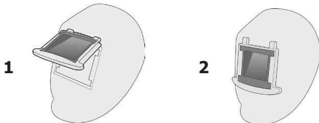
The FLIP-FLAP helmet can be used in two positions:
