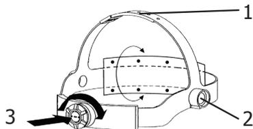
The FLIP-FLAP is equipped with a headband which can be adjusted in multiple ways to suit the welder: width, height (1), longitudinal inclination (3) and adjustment (2).
