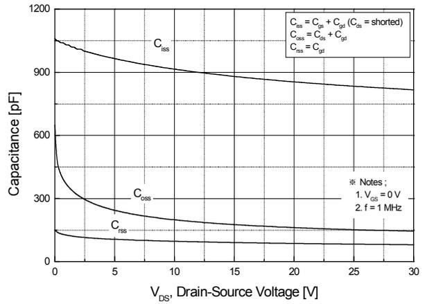
**Fig.8 Capacitance Characteristics**
