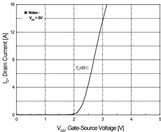
**Fig.5 Transfer Characteristics**
