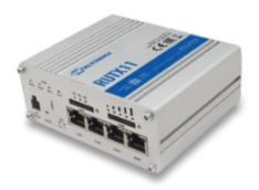
Most powerful and feature rich device within Teltonika Networking products range. Equipped with Dual-SIM, 4 x Gigabit Ethernet ports, Dual-Band AC WiFi, Bluetooth LE and USB interfaces. RUTX11 comes with all RutOS software and security features. This device is perfect for advanced Industrial and Enterprise applications.
