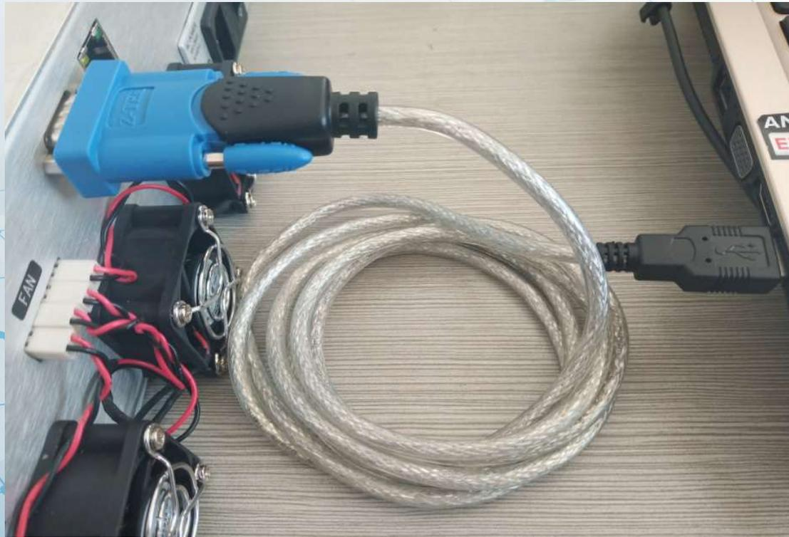
2.As shown in the figure, open EDFA, open computer client SSCOM software, select ComNum, click OpenCom and select Baud rate:19200.
