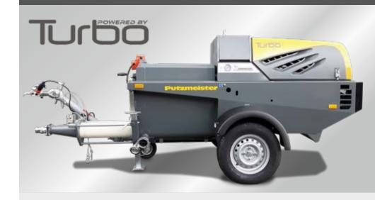
The SP 20 THF is a worm pump for self-levelling floor screed applications. Equipped with a 4 cyl. turbocharged Kubota diesel engine with 33 kW, this machine is more powerful and allows high delivery distances.
