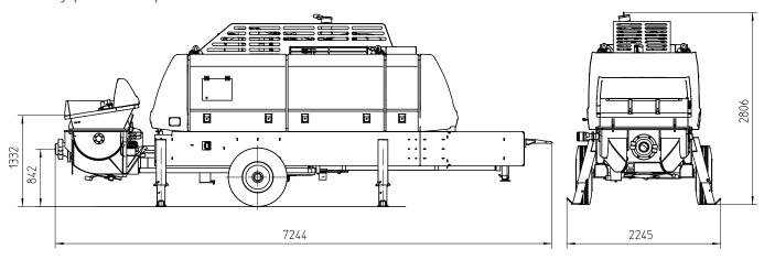
Note: Standard version BSA 2110 HP D5. Dimensions and weights depend on equipment. Subject to technical modifications and errors.
