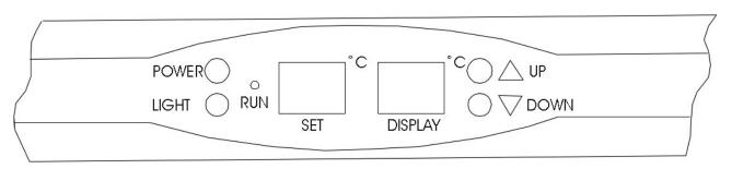
When the cabinet is turned on, the display will show the current temperature in the cabinet. SET displays set temperature.
