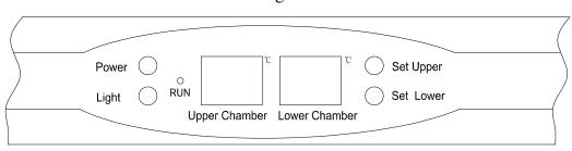
When the cabinet is turned on, the display will show the current temperatures in the cabinet's two chambers.
