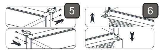
Move the hinge pin & washer to the opposite side. Mount the door and screws again.
