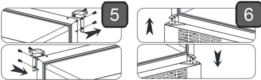
Move the hinge pin & washer to the opposite side. Mount the door and screws again.
