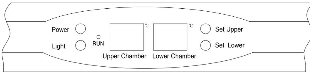
When the cabinet is turned on, the display will show the current temperatures in the cabinet's two chambers.
