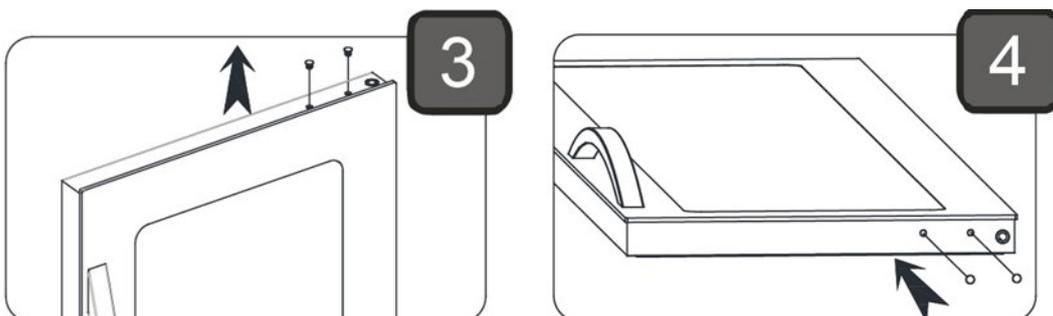
The enclosed top hinge should be fitted at the opposite side. Move the plastic support to the opposite side.
