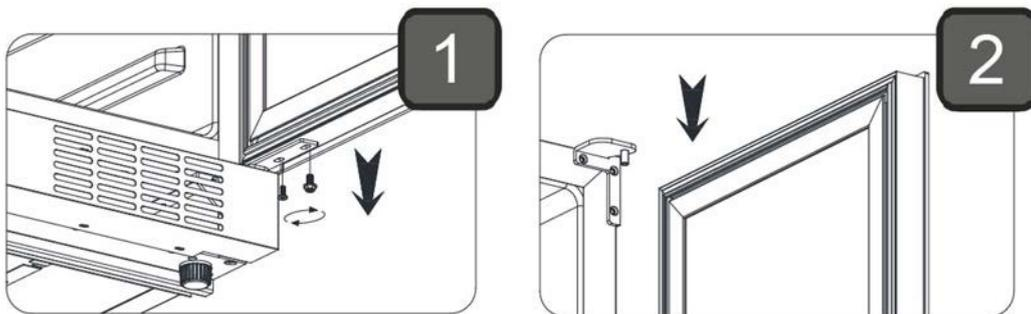
Move the two plastic caps from top to bottom and rotate the door 180 degrees. (Frameless)
