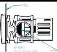
Instrument **XR02CX** shall be mounted on vertical panel, in a 29x71 mm hole, and fixed using the special bracket supplied. The temperature range allowed for correct operation is 0+60 °C. Avoid places subject to strong vibrations, corrosive gases, excessive dirt or humidity. The same recommendations apply to probes. Let air circulate by the cooling holes.
