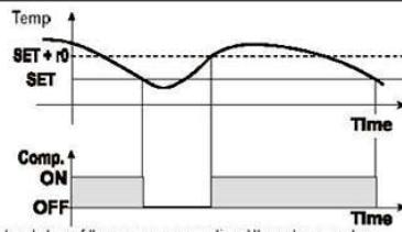
In case of fault in the thermostatic probe the start and stop of the compressor are timed through parameters "Cy" and "Cr".
