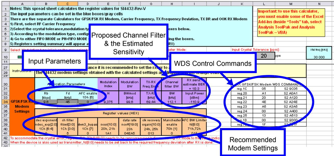
**Figure 7. Modem Parameters for FSK/GFSK Modulation**
