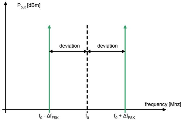
**Figure 4. FSK Modulation**
