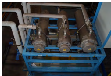
Picture 1: Pressure measurement at a flow pickling line for grease oils with Serv-Clip -1 and pressure sensor DS-1-A
