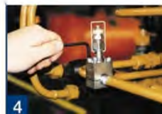
4 screw down clamp bolts
