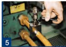
5 screw down clamp bolts
