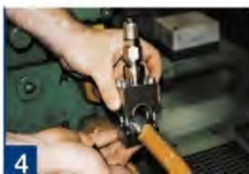
4 clamp SC onto pipe
