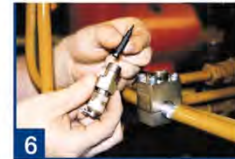
6 remove stirrup and needle
