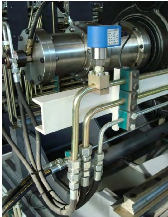
Picture 3: Leakage sensor with Serv-Clip -2 for recognizing seal damages at cylinders of a reeling machine
